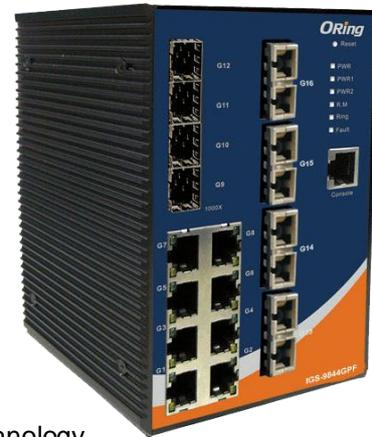
Featuring a wide operating temperature from -40°C to 70°C, the IGS-9844/9848GPFX series can be managed centrally and conveniently via Open-Vision, web browsers, Telnet and console (CLI) configuration, making it one of the most reliable choice for highly-managed and Fiber Ethernet power substation and rolling stock application
