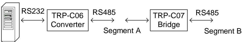
Now, you just need one TWIN485 box to support bridge function between RS485 segment A and segment B. And one PC COM port connect to TWIN485 box working in this RS485 network. In cost consideration you just need one TWIN485 box to replace TRP-C06 and TRP-C07 cost. From maintenance consideration you just need to have TWIN485 in stock.
