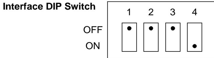
We need to set interface DIP SWITCH bit1,2,3 in OFF location and function DIP SWITCH bit1 in ON location.
