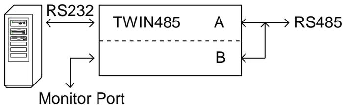
We can have one RS232 to RS485 converter circuitry as working unit. The other RS232 to RS485 converter circuitry as monitor and backup unit.
