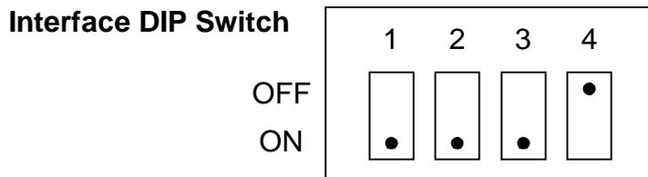
We need to set interface DIP SWITCH bit1,2,3 in ON location and function DIP SWITCH bit1 in ON location.
