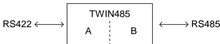
Normally RS422 is used in full-duplex point to point application. When you need to use such equipment in multi-drop environment, you need to change RS422 interface to half-duplex RS485 interface.
