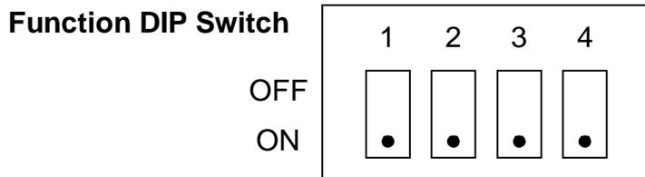
In this mode you can have two sets RS232 to RS422 converter to connect with RS422 devices.
