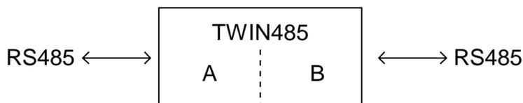
Normally RS485 network can cover 4000 feet range. When you need to cover over 4000 feet range, you need RS485 bridge.
