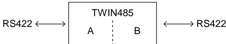
Normally RS422 can transmit upto 4000 feet. When you need to transmit over 4000 feet, you need RS422 repeater.
