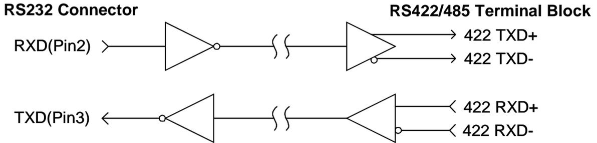
In Config. 1 is the signal relationship for RS232 interface and RS422/RS485 interface. Because RS422/RS485 interface is differential signal with plus signal name and minus signal name. And different company may have different meaning for such signal name. So user need to confirm the signal for TWIN485 box and other RS422/RS485 device.
