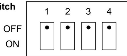
In this mode you can have two RS485 segment bridge in TWIN485.
