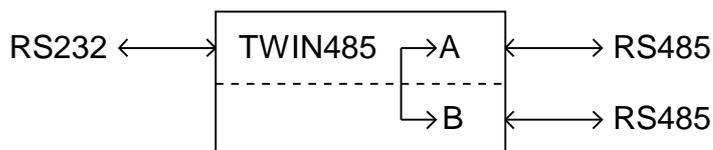
In this mode you can also set one interface to be RS422 type. So you can have one full duplex RS422 to half-duplex RS485 converter function.
