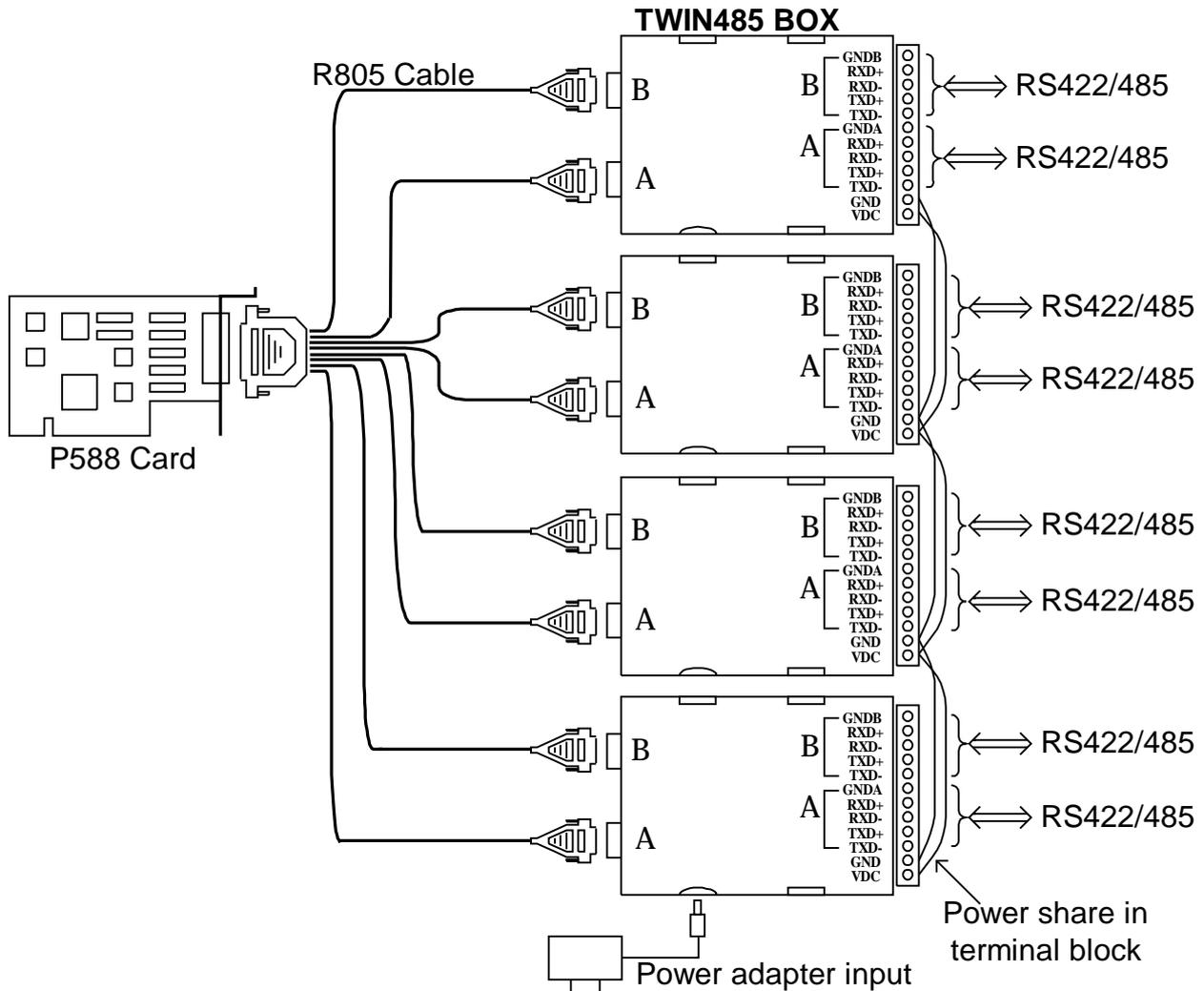
When you have our P588 card in your system, you can use one R805 cable to connect between P588 card and four TWIN485 boxes. Then you can have eight ground isolated RS422/RS485 port available.
