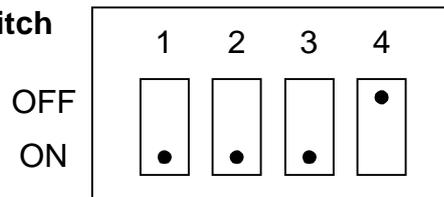
We need to set interface DIP SWITCH bit1,2,3 in ON location and function DIP SWITCH bit1 in OFF location.
