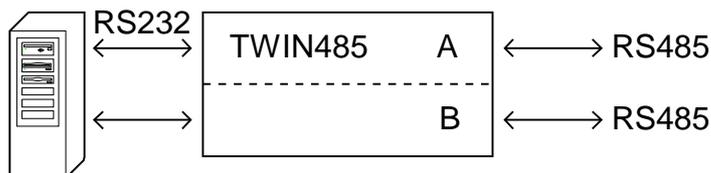
When we need to extend the cover range of RS485 network. We can have two RS485 segments. Each RS485 segment will cover 4000 feet range. So we can have two RS485 segments to cover 8000 feet range. In this application we will have two RS232 ports. Each RS232 port will use one RS232 to RS485 converter to handle one RS485 network.
