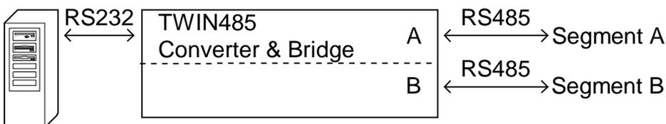
When we have one PC COM port to handle RS485 network. TWIN485 box set in BRIDGE mode is easy to use. But you need to have just one COM port to handle whole RS485 network, you may have some performance limitation. Because RS485 network is half-duplex structure. So one COM port need to poll each device and wait response.
