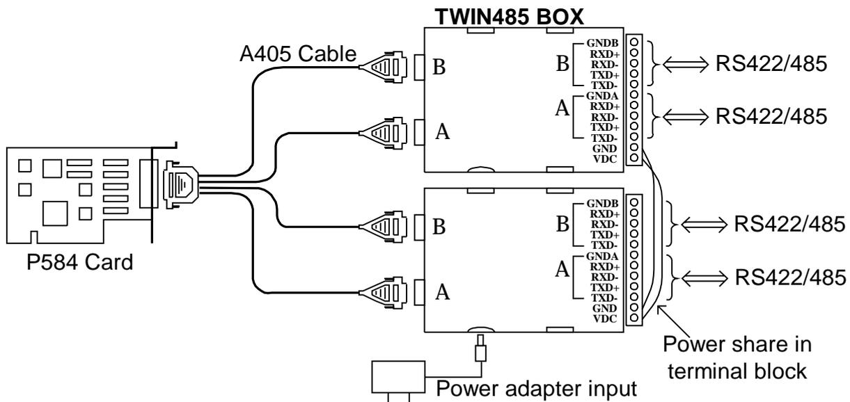
When you have our P584 card in your system, you can use one A405 cable to connect between P584 card and two TWIN485 boxes. Then you can have four ground isolated RS422/RS485 port available.
