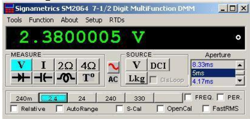
Figure 3-2. The Control Panel for the SM2064. The three main groups include Measure, Source and Range buttons. The Range buttons are context sensitive such that only “240m, 2.4, 24, 240 and 330 appear when in AC Voltage Function is selected, and 2.4m, 24m, 240m and 2.4 appear when AC Current functions is selected, etc.
