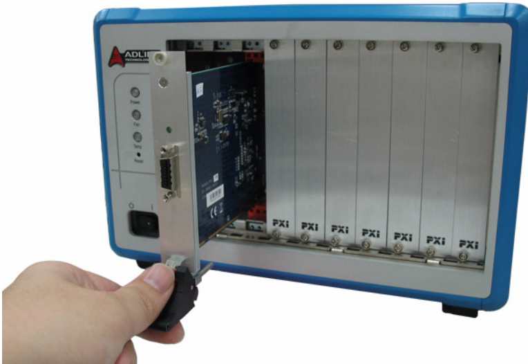
Figure 2-2: PXI-8565 to PXI™ Chassis Installation Diagram
