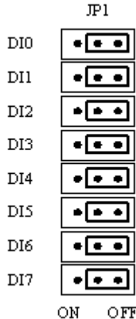
Figure 2-2: Default Input Signal Jumper Setting
