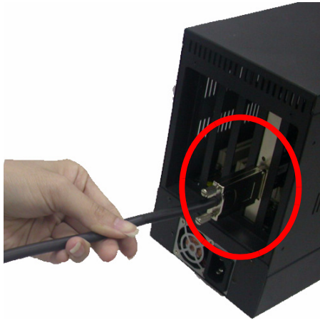
Figure 2-4: Cabling 3 M Extension Cable to Extension Chassis
