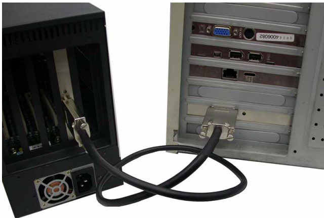
Figure 2-5: Host Computer connected to a PCI Extension System
