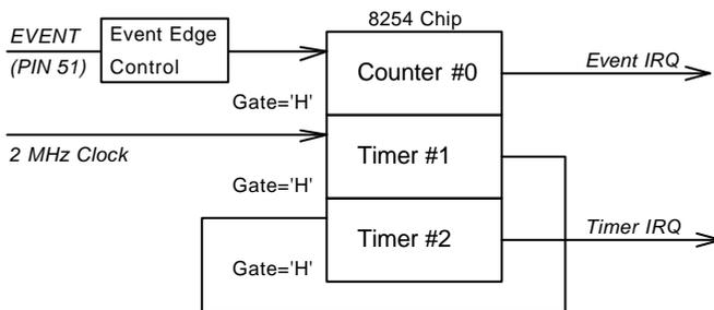
**Figure 4.3 Timer / counter system of PCI-7396.**
