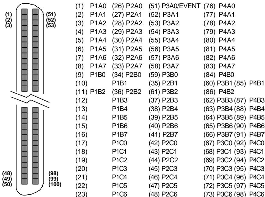
**Figure 2.3 Connectors Pin Assignment of PCI-7396**
