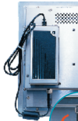
◀ New Power Module Mount on Rear Chassis
