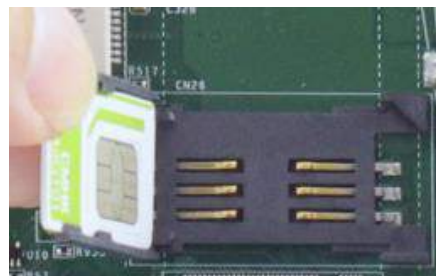
Insert SIM card with pins facing up
