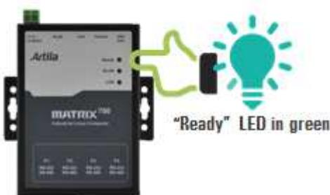
After completed above steps, the Matrix-700/710/713 will automatically reboot again when the backup process is finished.
