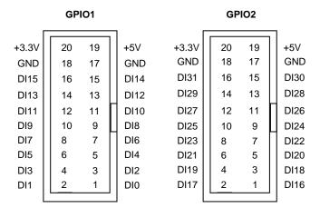
The signal level of GPIO is CMOS level and pitch of the pin header is 2.54mm. Each of the DIO pin can be programmed as digital input or digital output.
