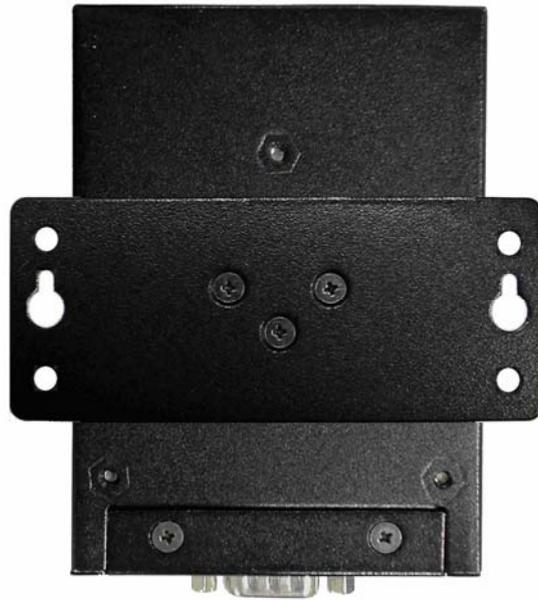
The screws specification shows in the following two pictures. In order to prevent IDS-3012 from any damage, the size of screws should not be larger than the size that used in IDS-3012.
