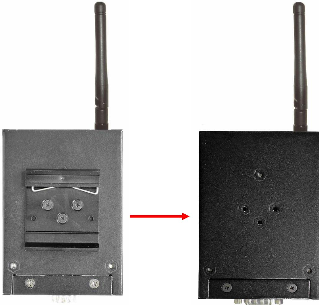
Step 2: Use 3 screws that can be found in the package to combine the wall mount panel. Just like the picture shows below:
