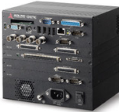
Figure 5-1: GEME w/one PMC and three PC-104 modules
