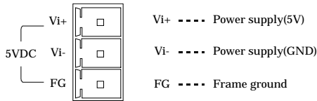
Figure 3.7. +5VDC Input Plug
