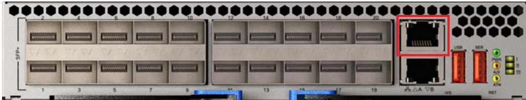
Figure 18: Connecting to LAN Port of COMe Module
