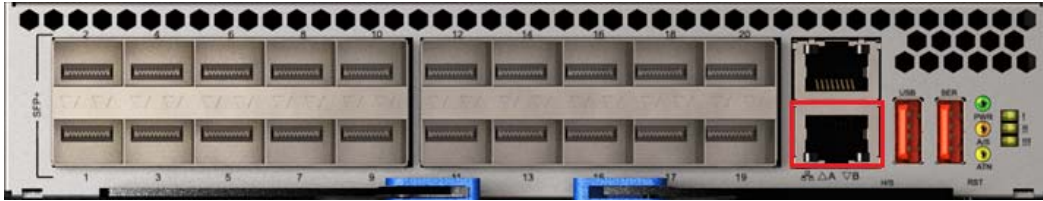
Figure 23: Connecting to LAN Port of CMM
